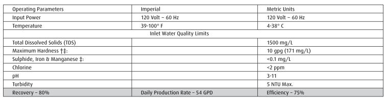
If the hardness of your water is above 10 gpg (171 mg/L), lime scale will build up rapidly on the membrane inside of the RO membrane cartridge. Scale build up will plug the RO membrane cartridge and make the system ineffective. We do not recommend the AquaTru® to be used with water in excess of 10 gpg (171 mg/L) hardness, unless the water is softened prior to the reverse osmosis system.
